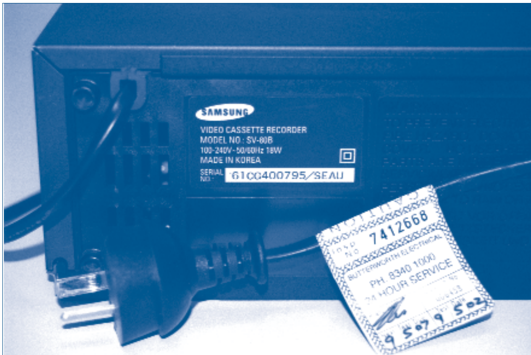
Example of a double insulated appliance (video player) with a 2-pin plug, square in square symbol and tagged in accordance with AS/NZS 3760
